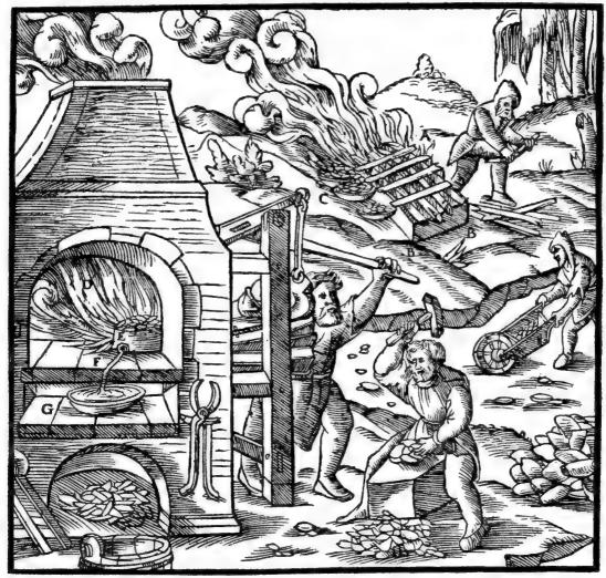
A-Wood. B-Bricks. C-Pans. D-Furnace. E-Crucible. F-Pipe. G-Dipping-pot.
